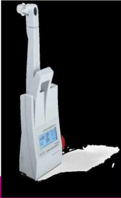
***Caption: The PASCAL's probe rests on the relaxed cornea with a constant force of one gram. Its piezoelectric sensor measures IOP 100 times per second.***
